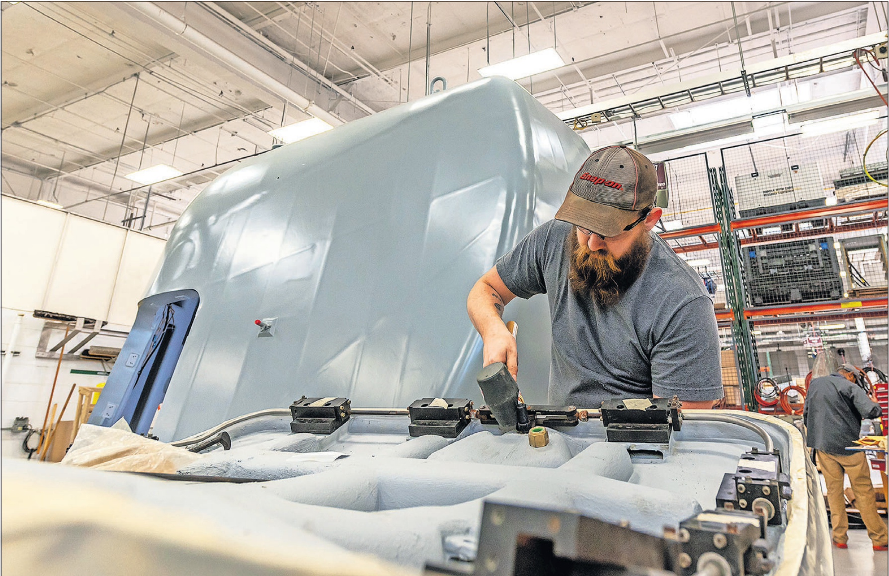
Industrial worker helper J.J. Johnson installs the locking mechanism for the weather shield door. The goal is to spend $65,000 and six weeks repairing each weather shield is assigned to the Systems Integration and Support Directorate's Electronics Shelter System Branch. [THOMAS ROBBIN/US ARMY PHOTO]
